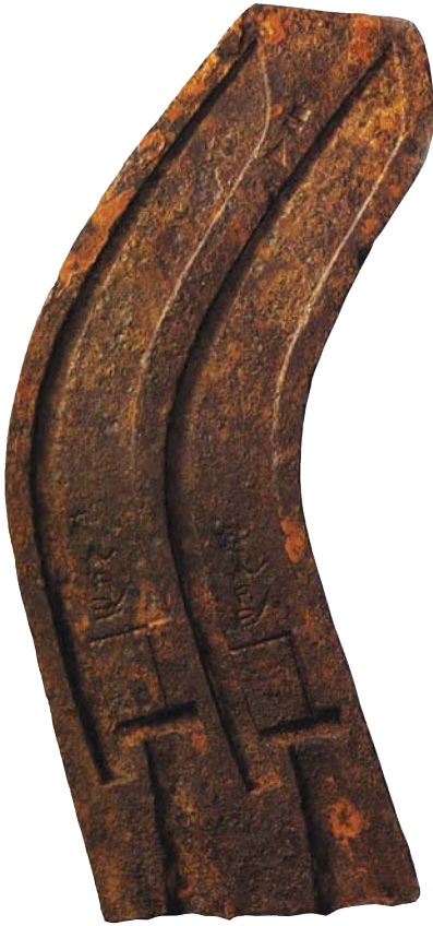
Mold for simultaneous casting of two iron sickles of the Warring States Period, unearthed in Gudonggou, Xinglong County, Hebei.
