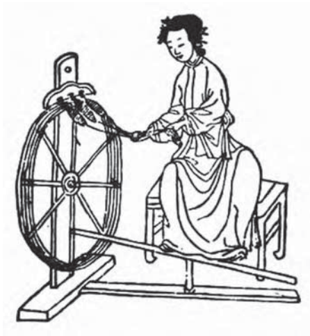
The cotton spinning wheel, an illustration from The Book of Agriculture by Wang Zhen of the Yuan Dynasty.
